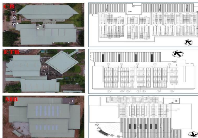
**Fig. 2 Layout of solar PV rooftop system**
