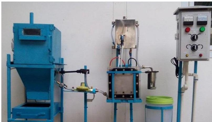
**Fig. 3 The Hydrogen Gas Incinerator Plant with 3 Sections**
